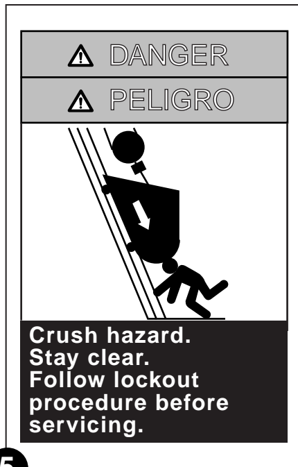
5 114688F0906 Crush Hazard Width 6 1/4 inch Height 9 1/2 inch
